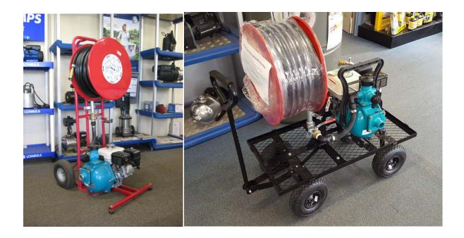
Our portable fire pump on a "sack truck" style trolley complete with hose reel is very popular. This gives the option of storing the pump and reel safely and out of the weather in the cooler months, which can then be wheeled into position ready for the fire season. As it is an "all-in-one" solution, it also saves installing a post to mount the hose reel.
