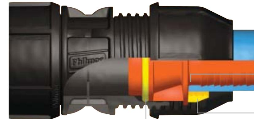
Insert fully installed into the pipe up to the shoulder of the insert.
